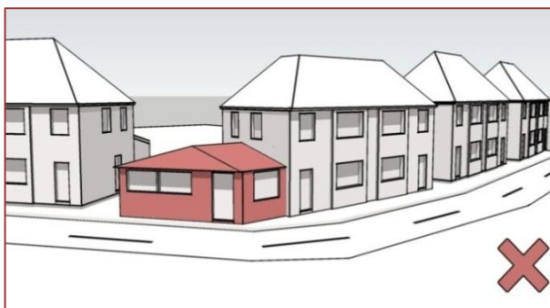
Figure 8 Side extensions on corner plots should be set back from the road and staggered where necessary
