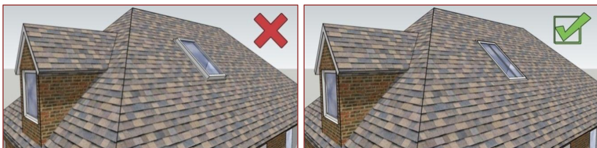
Figure 14 Inappropriate (left) and preferred (right) roof light designs
