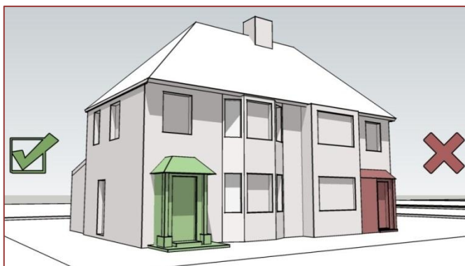
Figure 9 Front porches should not attach to the bay window
